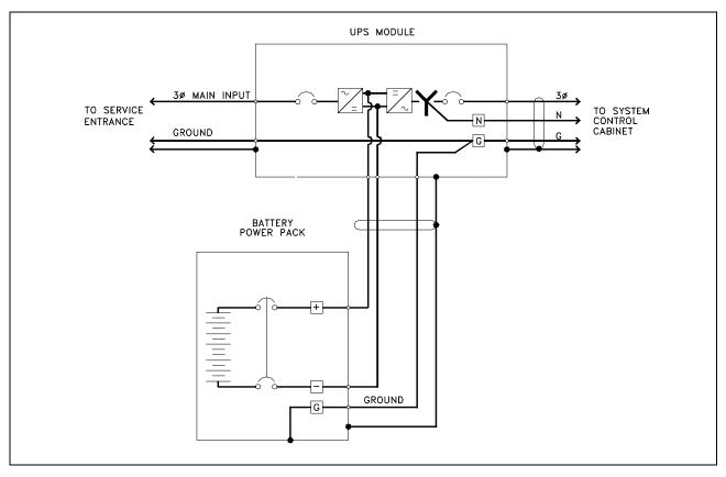
Large, open-rack battery systems are normally either locally grounded or left ungrounded, depending on local code requirements.
